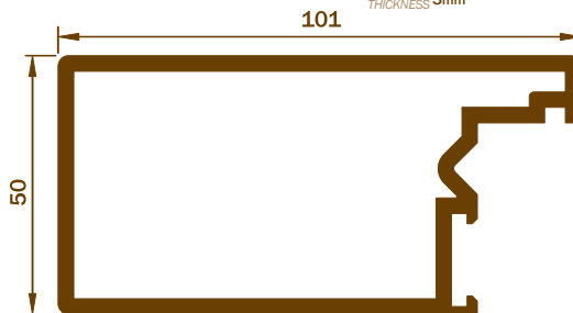
» HOJA PORTAL 101mm 101mm GATE SHEET REF. 2245 ESPEJOR THICKNESS 3mm
